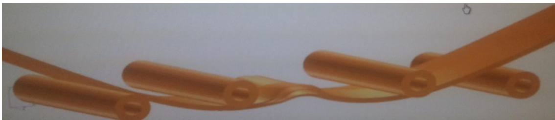
Figure 17. Deformed model showing delaminations
