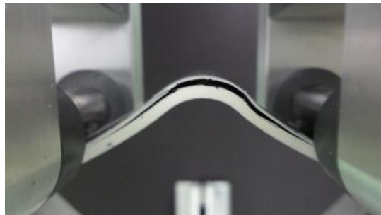
Figure 14. Example of Interlaminar Shear Failure
